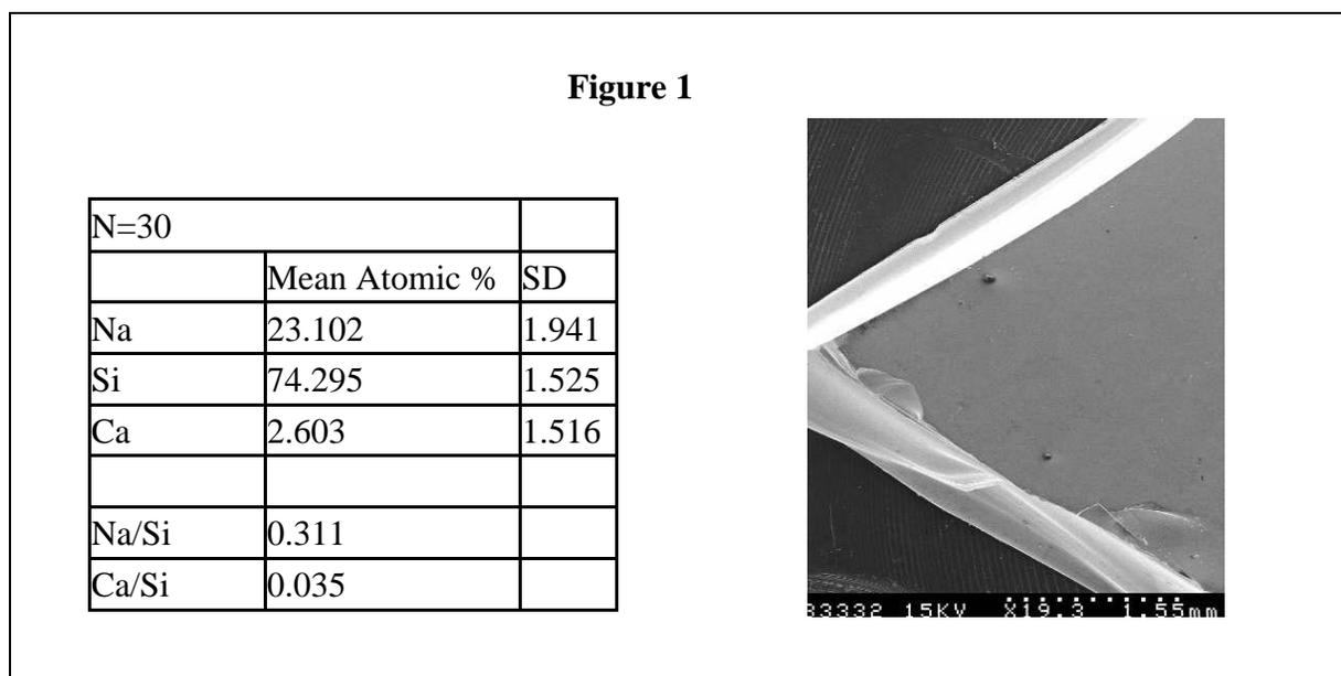
Elemental characterization following lead-rum exposure in the first batch of trials showed fairly erratic results. Lead was not present on the glass surface in the majority of the analyses.
