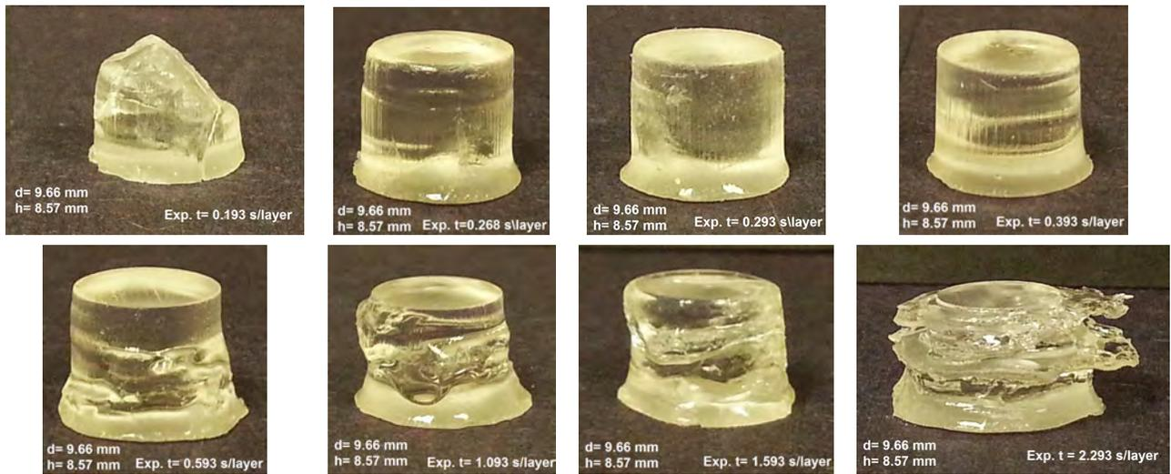
Figure 6: The results of a range of exposure times for Resin 1.0 and Resin 1.1. Evidence of overexposure becomes clear at  $t=0.593$  s/layer and becomes more dramatic as the exposure time is increased.
